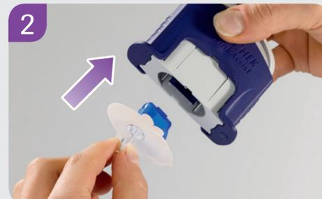
**2** Insert the infusion set from below into the loading chamber until it locks into place.
