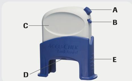
**A** Release button    **D** Loading chamber
